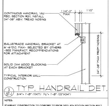
STAIRWAY CONSTRUCTION TO CONFORM TO FBCR 2023, 8TH EDITION SECTION R311.7
