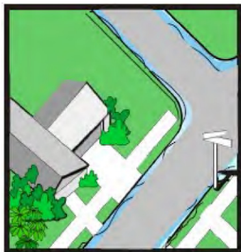
Service Level A FLOW CONTAINED WITHIN SYSTEMS
