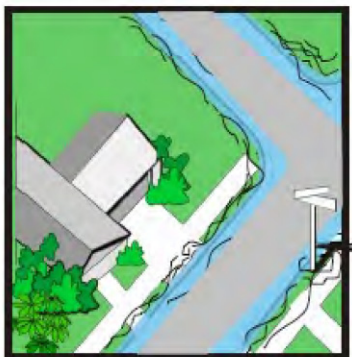
Service Level B WATER CONTAINED WITHIN RIGHT-OF-WAY
