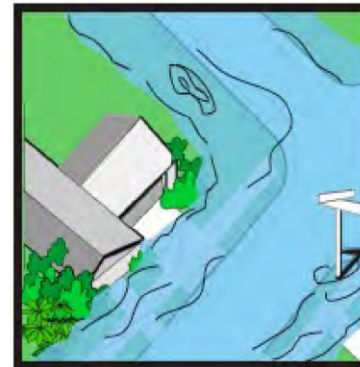
Service Level C WATER CONTAINED WITHIN FRONT YARD
